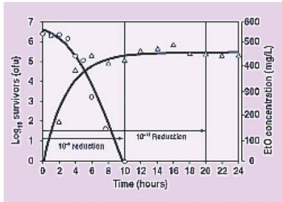
Figure 3. EtO concentration was mapped over a 24-hour cycle time. This graph depicts 10 degrees of lethality correlated to product level gas concentration and time at a constant process temperature.
